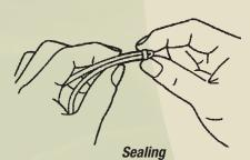
Place sealing clip onto folded tubing.
