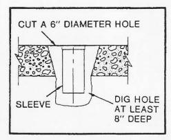
When the cement-in sleeve is to be installed in an existing concrete floor or deck, a hole at least 6-inches in diameter must be cut. The opening must be at least 8-inches deep. Fill the bottom of the hole with a non-shrinking cement, such as Por-Rok. Make sure the sleeve is perfectly vertical. Fill in around the sleeve with more non-shrinking cement. Allow the cement to set-up and finish the top surface.
