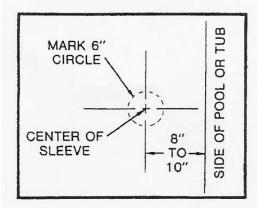
The layout required for the cement-in sleeve is shown on the diagram to the left. Proper position for the mast is 8 to 10 inches from the edge of the pool or tub. The cement-in sleeve itself is a cylinder 31/4-inches in diameter and 8-inches long. Mark a 6-inch circle if existing concrete is to be removed. In a new installation, position the sleeve on center and flush with grade.
